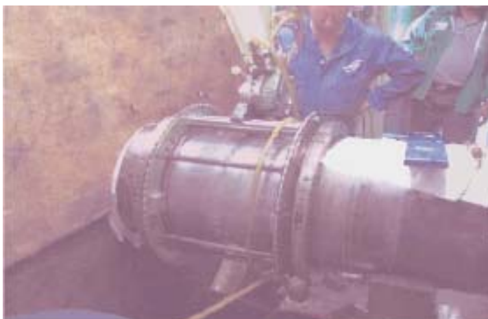
The orbital turning machine, designed and manufactured by Metallock Eng UK, rotates the tool around the shaft instead of the shaft being revolved past a stationary tool.
