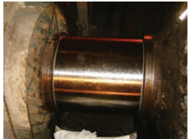
After machining to clean-up using orbital turning techniques
