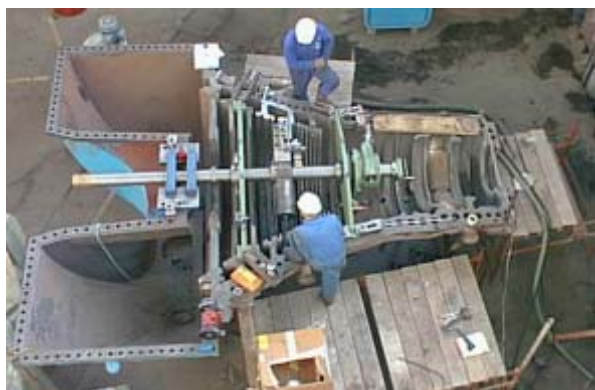
Machining to remove the four rows of blades on the turbine casing cover was done in an adjacent bay by using a cooling system to cut away the centre of the existing caulking pieces without cutting into the serrations.
